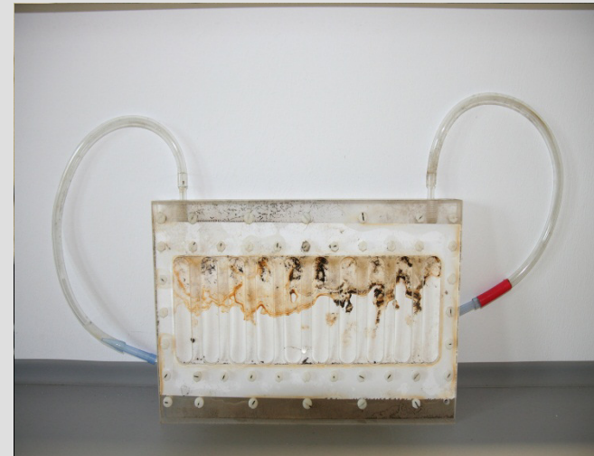
Rechargeable sampler for lab and field experiments to monitor temporal concentration changes (Zak & Gelbrecht 2007)
