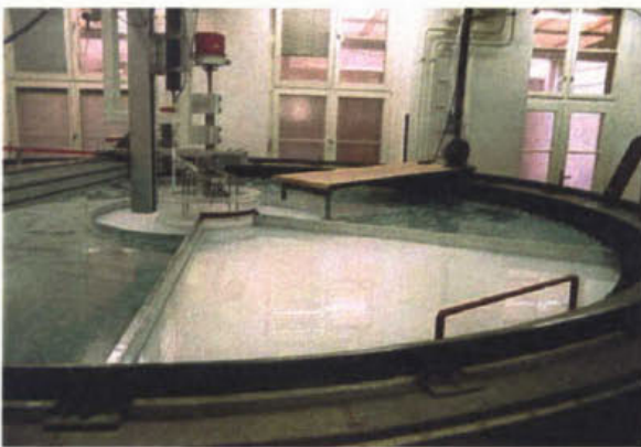
c) Test Measurement with the Moving Bottom Device in a sector of the Tank.
