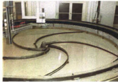
b) Five Scrapers with higher Scraper Blades and an increased Length
