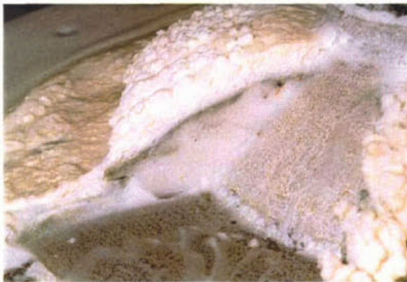
a) Lewatit particles sticking at the inlet of the model
