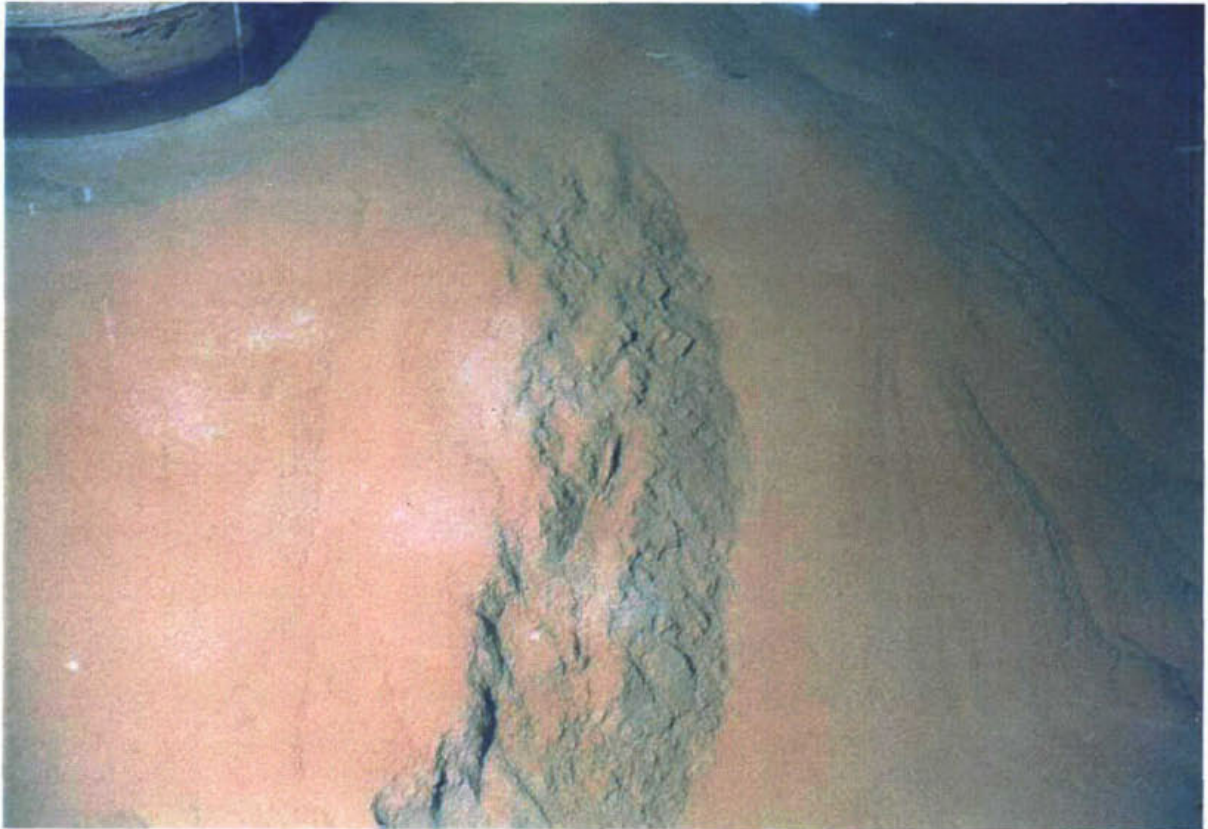
Fig. 6.3 Also with Iron Hydroxide the System fails due to separation of Lewatit and Flocks.
