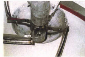
c) Detail of the Inner Support of the Scrapers (Changed later due to too high friction)
