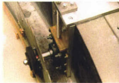
e) Inner Part of the Drive. First Version with a Friction Wheel
